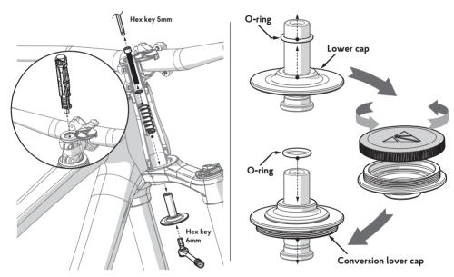
3. Insert the tool housing into the steerer tube and loosen the stem bolts. Make sure the top cap bolt is on the right-hand side.
