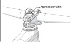
4. Measure the stack height between the top of stem to bottom of fork crown. Choose the proper M6 bolt according to the table below.
