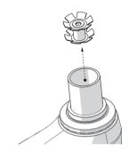
3. Put the stem and spacers onto the steerer tube. Make sure the steerer tube is lower than the top of stem or spacer by about 3mm.
